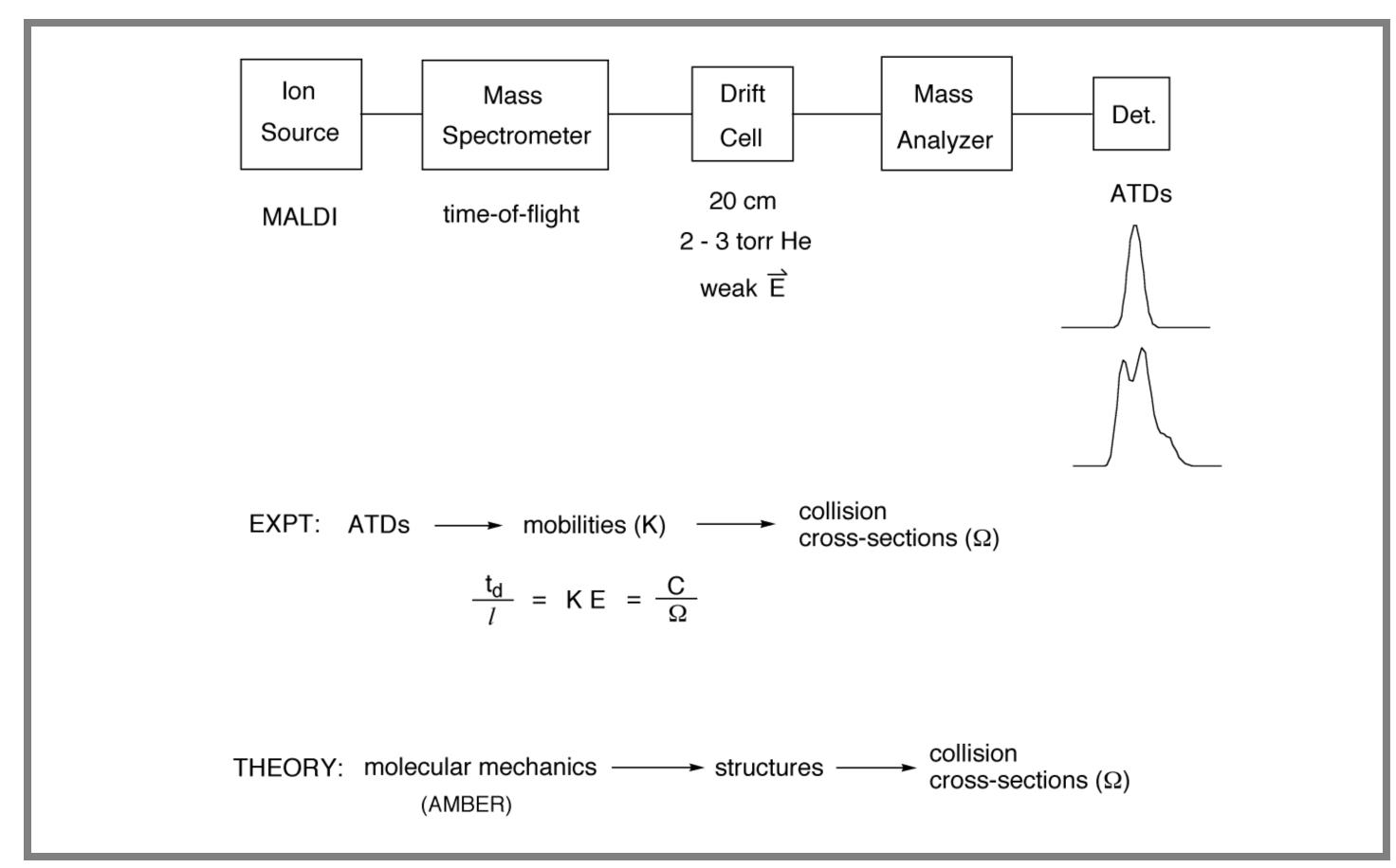
Matrix Assisted LASER Desorption/Ionization and Time of Flight Mass Spectrometer
